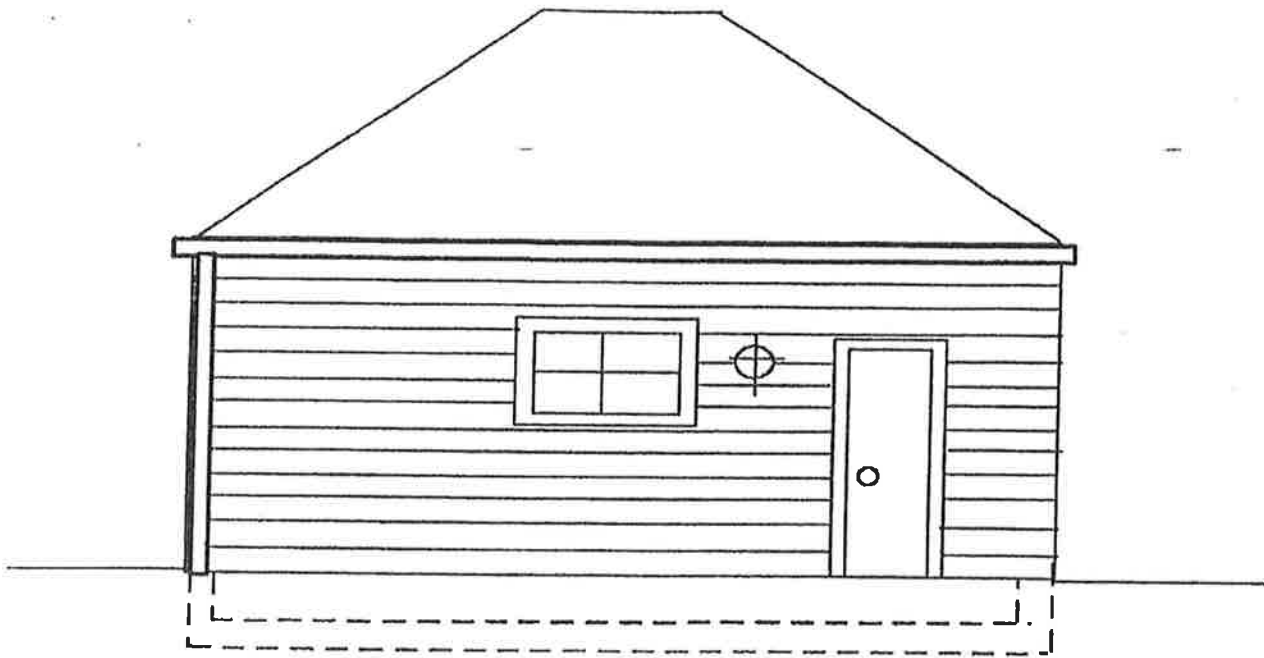
Side Elevation Detached Garage
